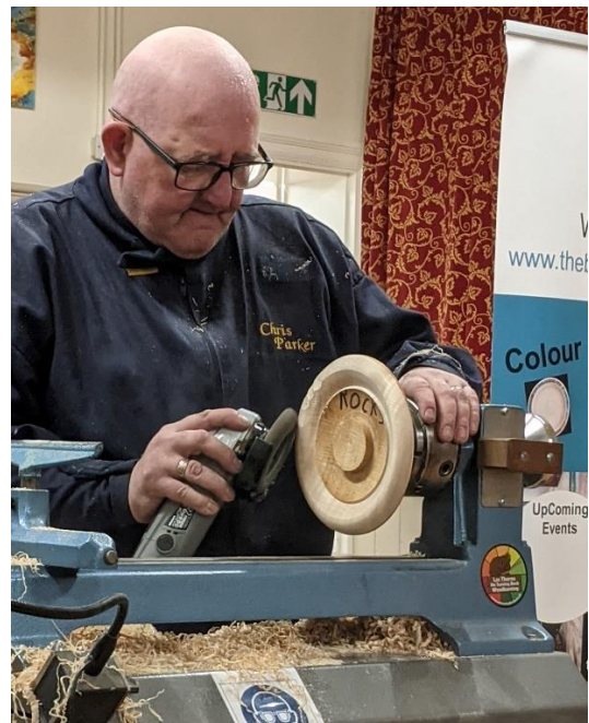
Use of a micro-motor or angle grinder to decorate the rim of a bowl before hollowing.
