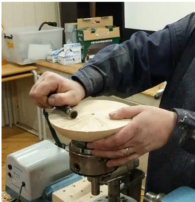
Use of a micro-motor or angle grinder to decorate the rim of a bowl before hollowing.
