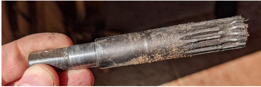
Damaged gear teeth on right hand side
